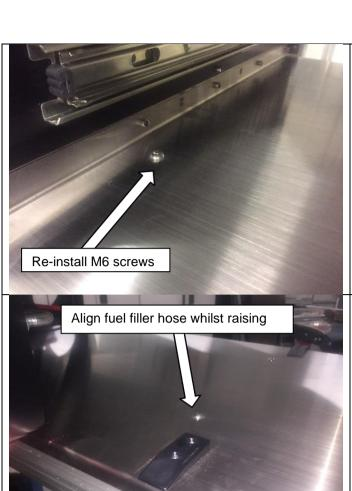
Re-install the M6 screws and flange nuts to the lower kitchen panel behind the drawer face.
