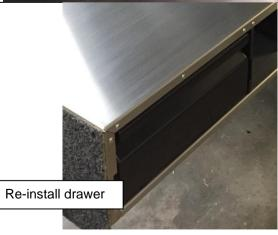
Carefully align the drawer runners on the small drawer, then push the drawer back to the red drawer latch. Rotate the latch down and push the drawer all the way in to reset the runners.
