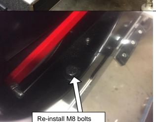
Re-install the M8 bolts with a washer under the head inside the hinge box. Install the M8 nuts to the underside.
