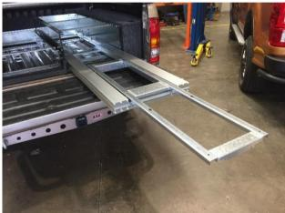
Fully extend the trolley ready to accept the kitchen assembly.
