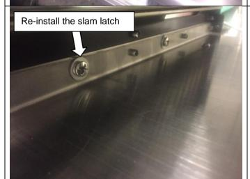
Re-install the drawer slam latch to the front face of the drawer, using the 4 screws with washers removed earlier.
