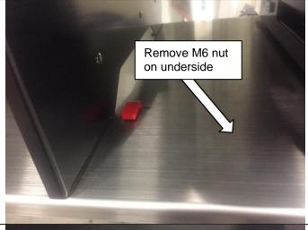
Before installing into the vehicle, the kitchen module must be removed from the cabinet.
