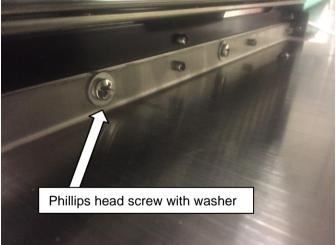
Remove the drawer slam latch from the front face by removing the 4 phillips head screws with washers under the heads located behind the front face.
