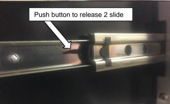
Remove small drawer by pushing the red drawer latch to the side and pulling out the drawer. Then push black lever on each drawer slide. Note, one lever is to go up and one lever is to go down. Pull the drawer out once the lever is depressed.
