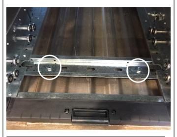
At this point, refer to the vehicle specific side floor kit installation instructions for the appropriate details on hat mounting positions on the base of the cabinet.
