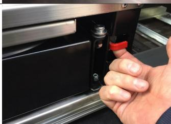
Open the swing out hob by pulling the red release lever near the hinge, with your other hand swing out the hob.
