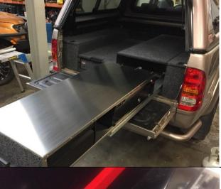
Using 2 people place the kitchen assembly onto the inner trolley.
