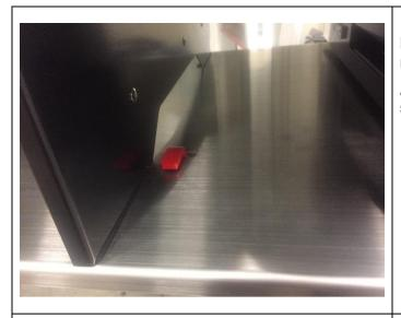
Re-install 2nd stage lock out lever by placing the lever over the M6 bolt and securing with the M6 nylock nut on the lever pivot.
